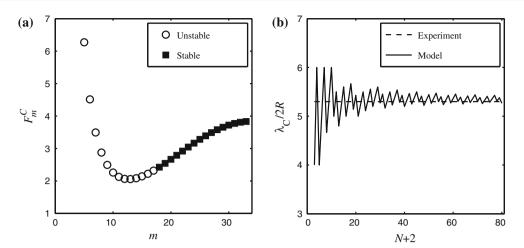
**Fig. 4** Model predictions for P1 parameter set and  $R = 1.6 \,\mu\text{m. a}$  Critical buckling loads for N + 2 = 35 ( $F_{min}^C = 2.06$  N and  $m_{min} = 13$ ). **b** Predicted critical wavelengths consistent with those observed in exper-
