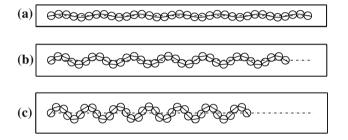
Fig. 7 AUTO generated post-buckling configurations for increasing strain along least energy solution branch emanating from  $m_{min} = 13$  with parameter set P1,  $R = 1.6 \,\mu\text{m}$  and N + 2 = 35: **a**  $\varepsilon = 1.35 \,\%$ , **b**  $\varepsilon = 10 \,\%$ , **c**  $\varepsilon = 25 \,\%$
