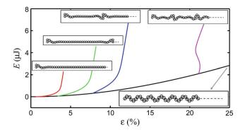
**Fig. 6** Energy of post-buckling configurations generated by AUTO for increasing strain emanating from  $m_{min} = 13$  with parameter set P1,  $R = 1.6 \,\mu\text{m}$  and N + 2 = 35. Sinusoidal modes are energetically favoured; bifurcations which lead to localisation are marked by an increase in potential energy
