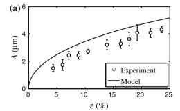
**Fig. 8** Comparison between model predictions of **a** amplitude and **b** wavelength (parameter set P1,  $R = 1.6 \,\mu$ m and N + 2 = 35) with one representative realisation of experimental measurements: compare
