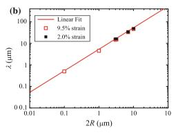
Fig. 2 Typical experimental results. **a** Wavelength  $\lambda$  scaled by particle diameter 2*R*, for several different colloidal samples on identical substrates. The average slope extrapolates to a zero strain wavelength of 5.3  $\pm$  0.4. Note the linear relation at small to moderate strain. No
